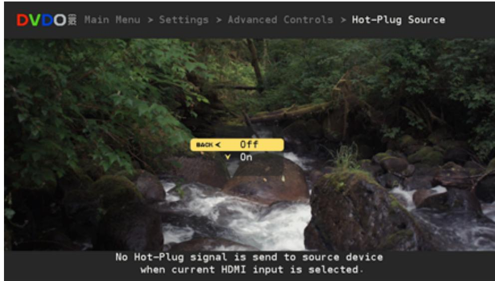
To enable Hot Plug Source, first select an HDMI input, then go to the menus to the window shown above, and select “ON.”
