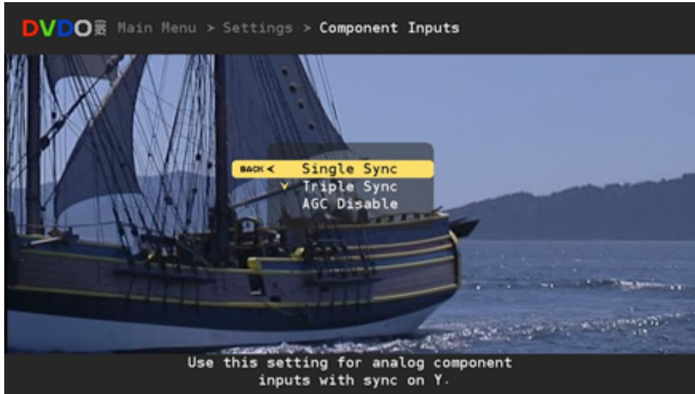
The Component Inputs window gives you 3 options for controlling Automatic Gain Control on Analog Inputs:
