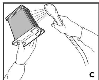
**D.** Remove the lint from the heat exchanger housing by hand or with a damp cloth. Clean the entire housing from the back to the front side, ensuring that all lint is removed.
