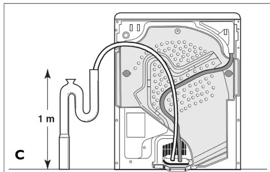
**Notice:** To prevent water siphoning back into the appliance, the end of the hose must not be immersed in the drain water. Avoid bending and twisting the hose.
