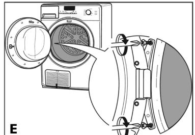
**NOTE:** Ideally you should use a Torx T20 type screwdriver to undo and tighten the screws.
